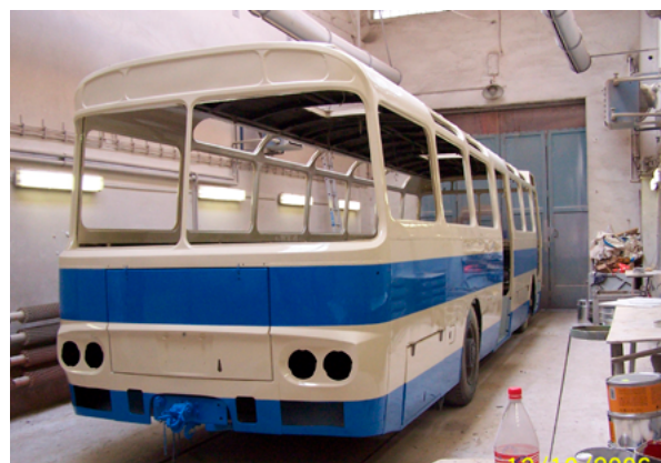
10. Lakiranje autobusa Karosa ŠL 11.1305 u centralnoj radionici Gradskog prometnog poduzeća u Brnu. Autobus je premazan krem bojom nijanse RAL 1015 s dva plava pojasa nijanse RAL 5015 (TMB, snimka: T. Kocman, 2006.) Varnishing of the Karos ŠL11.1305 bus in the central workshop of the City Transport Company in Brno. The bus was coated with cream-coloured paint, shade RAL 1015, with two blue bands, shade RAL 5015 (TMB, T. Kocman, 2006)
