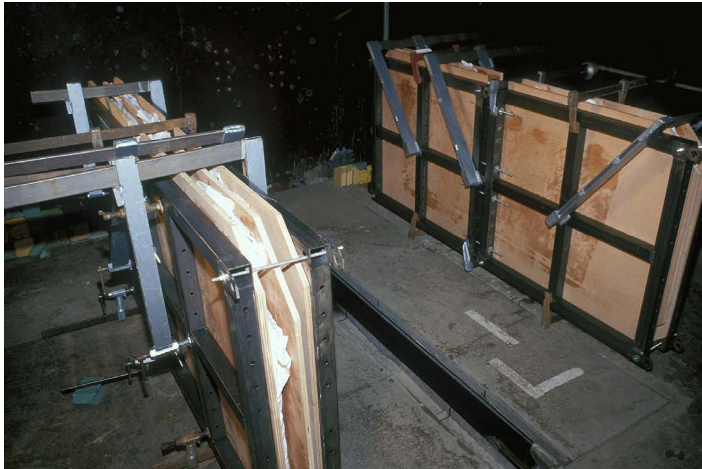
Parquet pannels in their support inside the irradiation chamber
