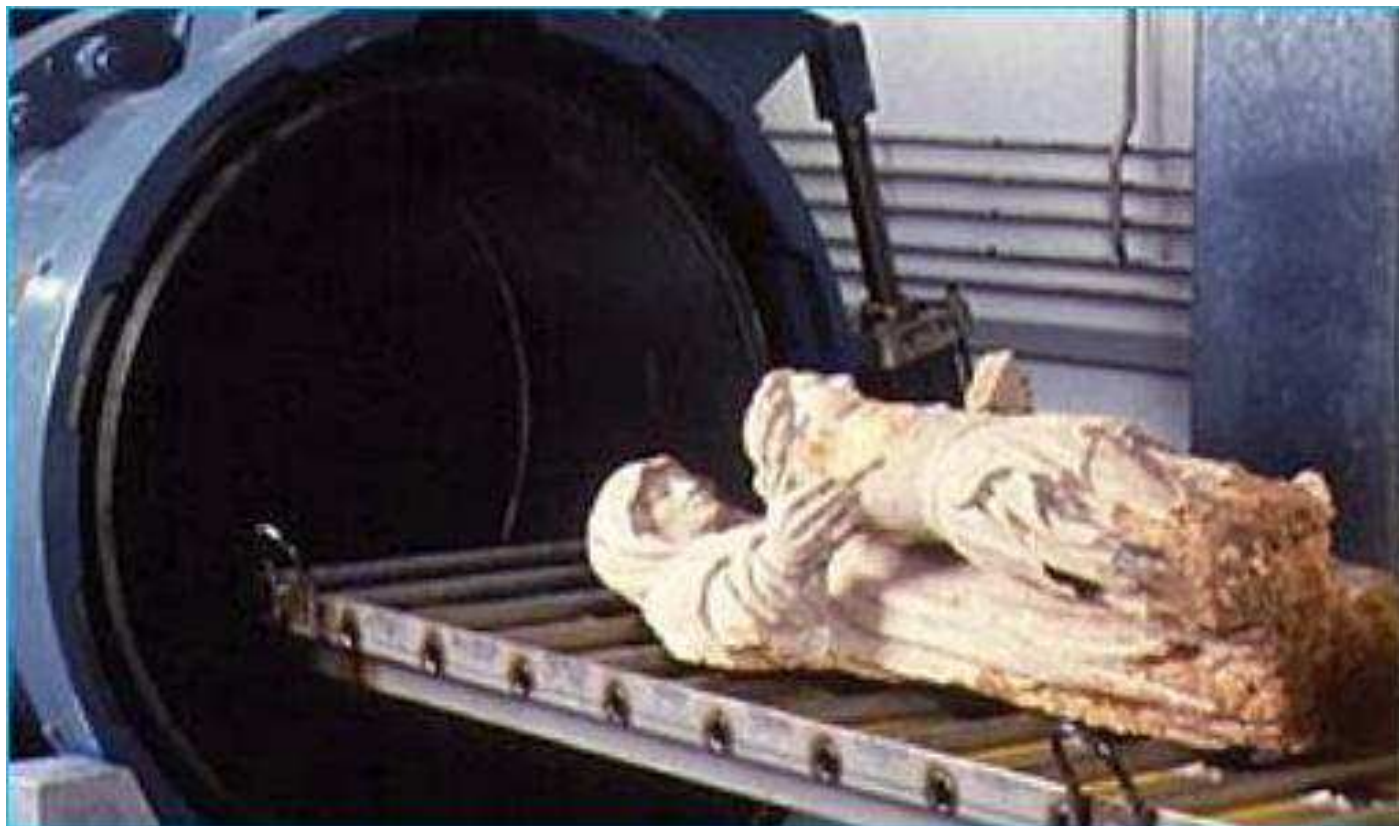
Impregnation tank (vacuum/pressure) 1000 litres
