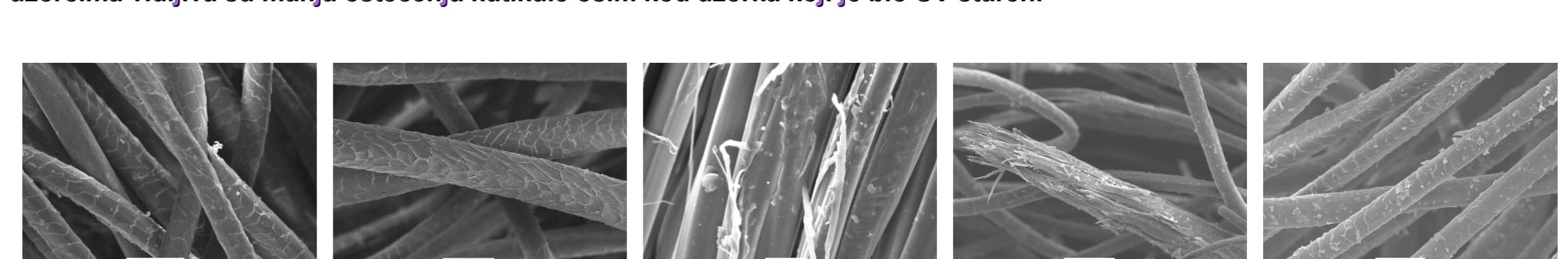
SEM mikrografs of unaged and aged wool samples: unaged and unirradiated (left), aged and unirradiated (center left), unaged and irradiated 120 kGy (center), aged and irradiated 120 kGy (center right), UV-aged and irradiated 120 kGy (center right). Slight damage of cuticule is visible in irradiated samples except the UV-aged one.
