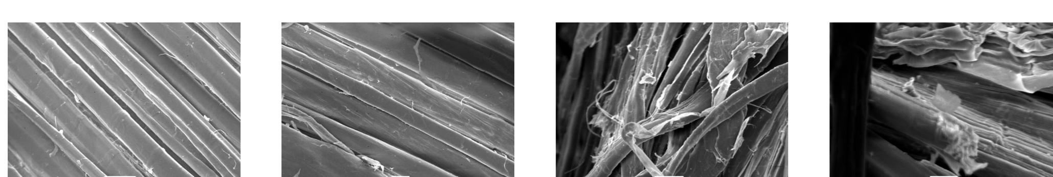
SEM mikrografs of unaged and aged cotton fibers. The first two images show unaged and aged cotton respectively. The third and fourth images show unaged and aged cotton fibers irradiated with 120 kGy. Labels indicate X500 and X1000 magnification.
