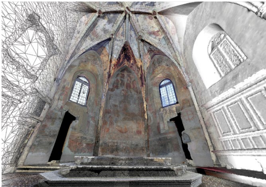
| Church of St. Nicolas in Pazin - Orthophotos of wall paintings integrated in 3D model of the church interior acquired with several 3D scanning techniques (Vektra d.o.o.) Crkva sv. Nikole u Pazinu - ortofoto zidnih slika integriran u 3D model unutrašnjosti crkve dobiven korištenjem nekoliko tehnologija 3D skeniranja (Vektra d.o.o.)
