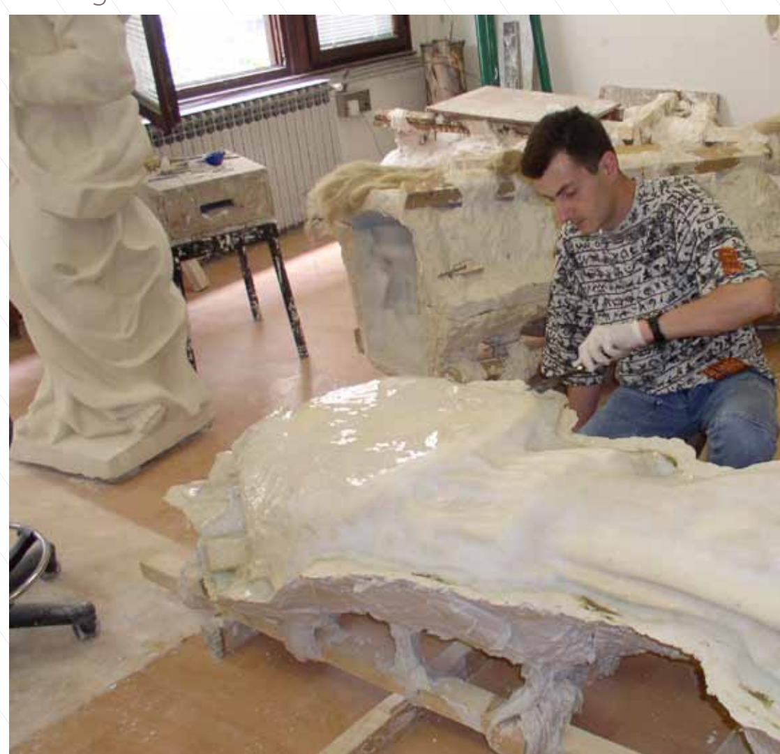
Izrada kalupa Making of the mould
