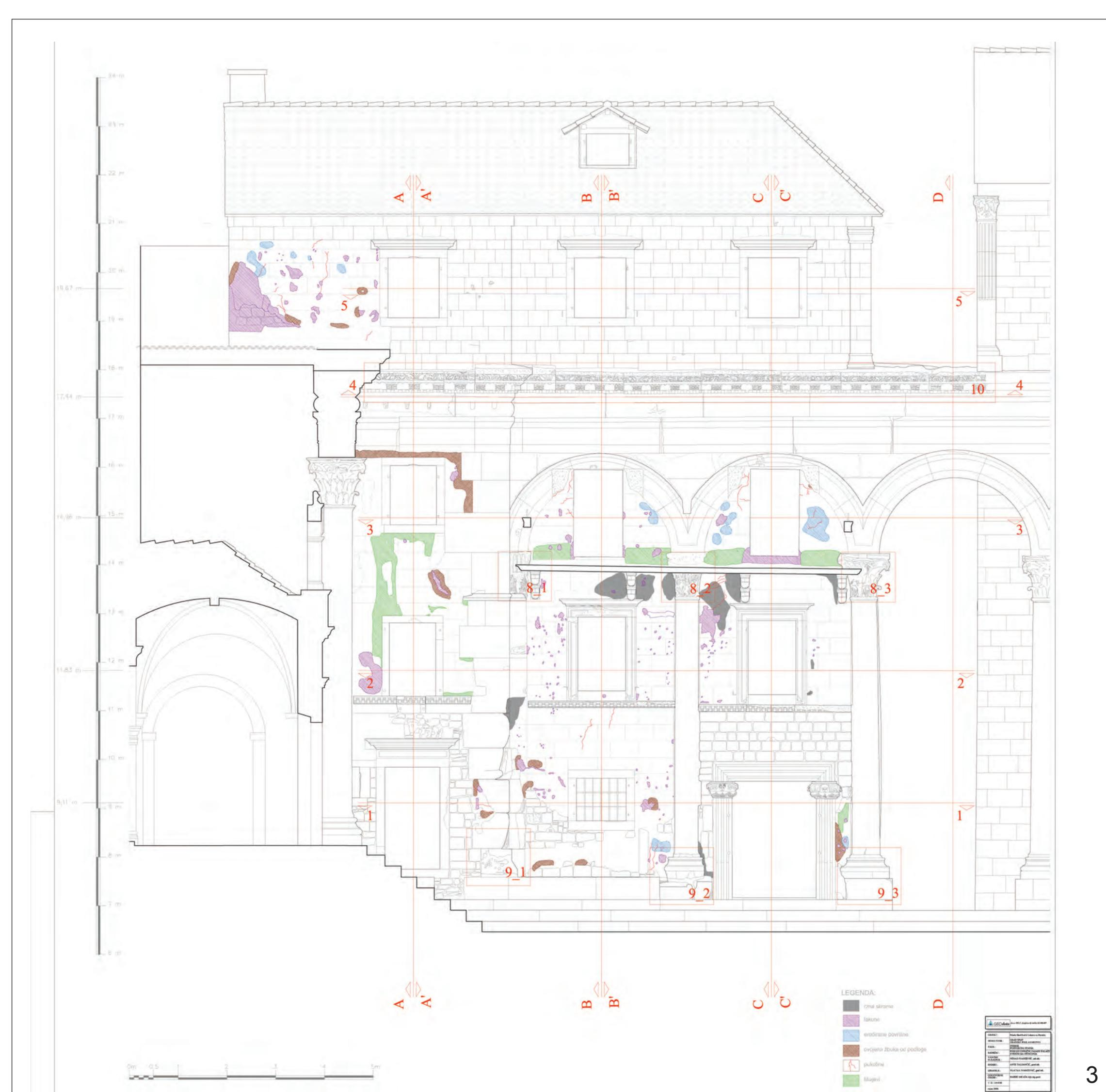
At the beginning of August 2006 scaffolding was put up in the south west corner of the square. An architectural drawing of the southern part of the western colonnade and the façade of the Skočibučić-Lukaris Palace (Fig. 1) was made, and the drawing obtained was used as a base for the precise recording of damage and impurities (Fig. 2, Fig. 3). As well as in the drawing, the situation as found was documented with photographs and written reports.
