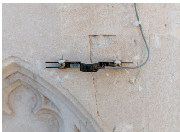
12. Orlando's Column, pillar, east side, sensor for measuring the displacement of cracks (HRZ Archive, P. Gamulin, 2021)
