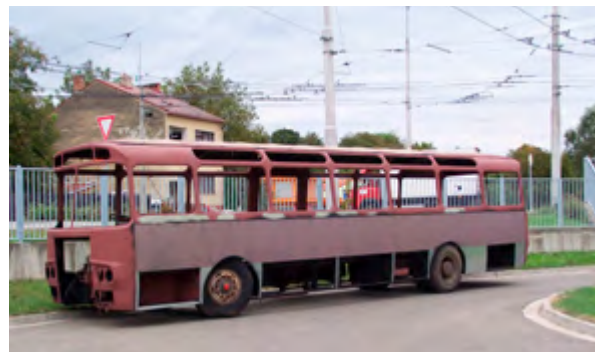
8. U listopadu 2006. godine u garaži Komín prijevoznog poduzeća grada Brna, završeni su konzervatorsko-restauratorski radovi na kosturu kolnog ormara autobusa Karosa ŠL 11.1305 (TMB, snimka: T. Kocman, 2006.) Conservation of the frame of the coachwork of the Karos ŠL 11.1305 bus was completed in October 2006, in the garage of the Komín transport company of the city of Brno (TMB, T. Kocman, 2006)
