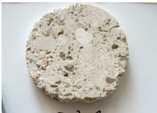
16. Standardizirani testni uzorak srednjovjekovnog arriccio (snimio B. Hacker, 2009.) Standardized test sample of the medieval arriccio (photo by B. Hacker, 2009)
