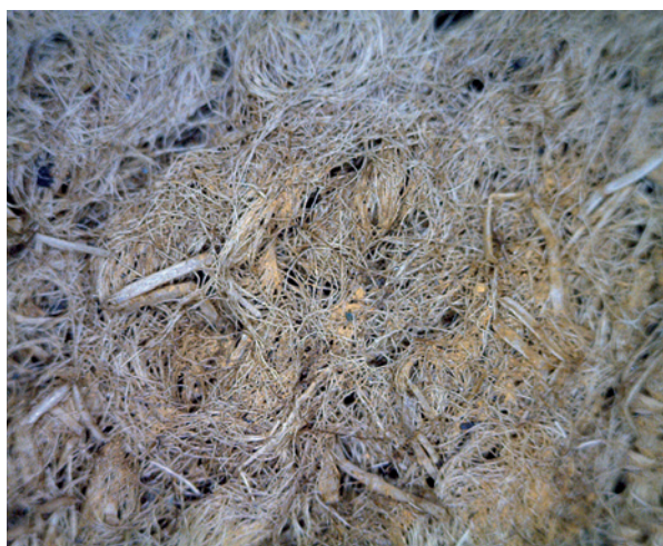
9d. Mikroskopski snimak (56 x) uzorka efekta valjane tkanine (fototeka HRZ-a, snimila K. Hrepić) Microscopic image (56x) of the sample effect of fulling of the fabric (Croatian Conservation Institute Photo Archive, photo by K. Hrepić)
