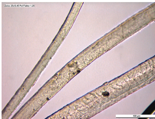
11. Transmitted light microscopy: left: sheep wool; right: flax. Samples from the salt-mine Hallstatt (photo: K. Grömer, © Natural History Museum Vienna).
