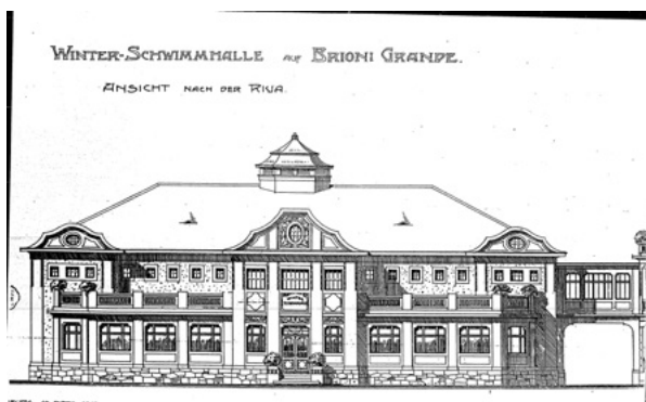
11. Eduard Kramer, nacrt glavnog pročelja zgrade zimskog bazena, 1911. (Odjel za kulturnu baštinu Javne ustanove NPB) Eduard Kramer, plan of the main façade of the indoor-swimming-pool building, 1911 1910 (Brijuni National Park Subdepartment for Protection of Cultural Heritage)
